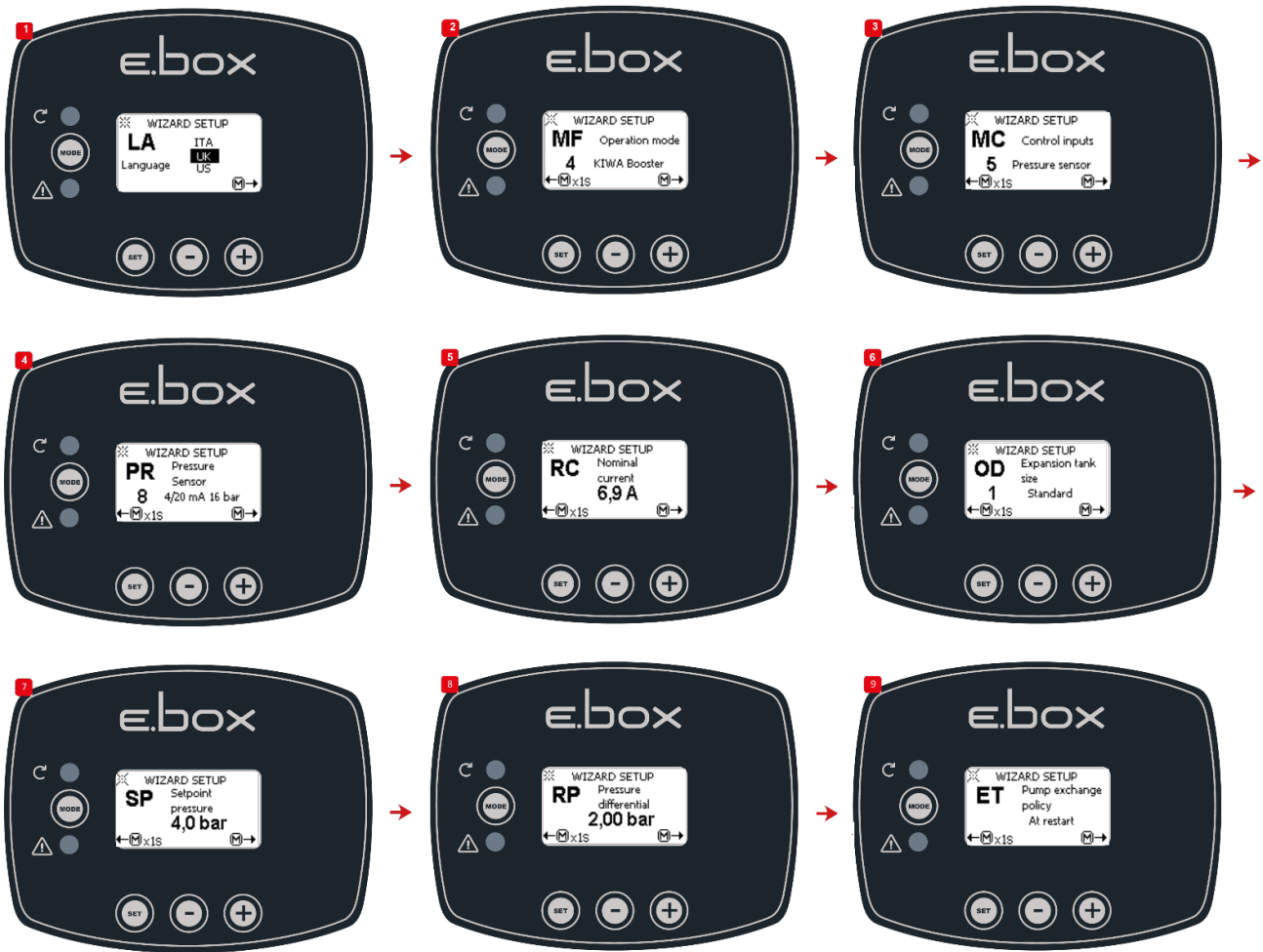
Figure 48: KIWA pressure boosting with pressure sensor
