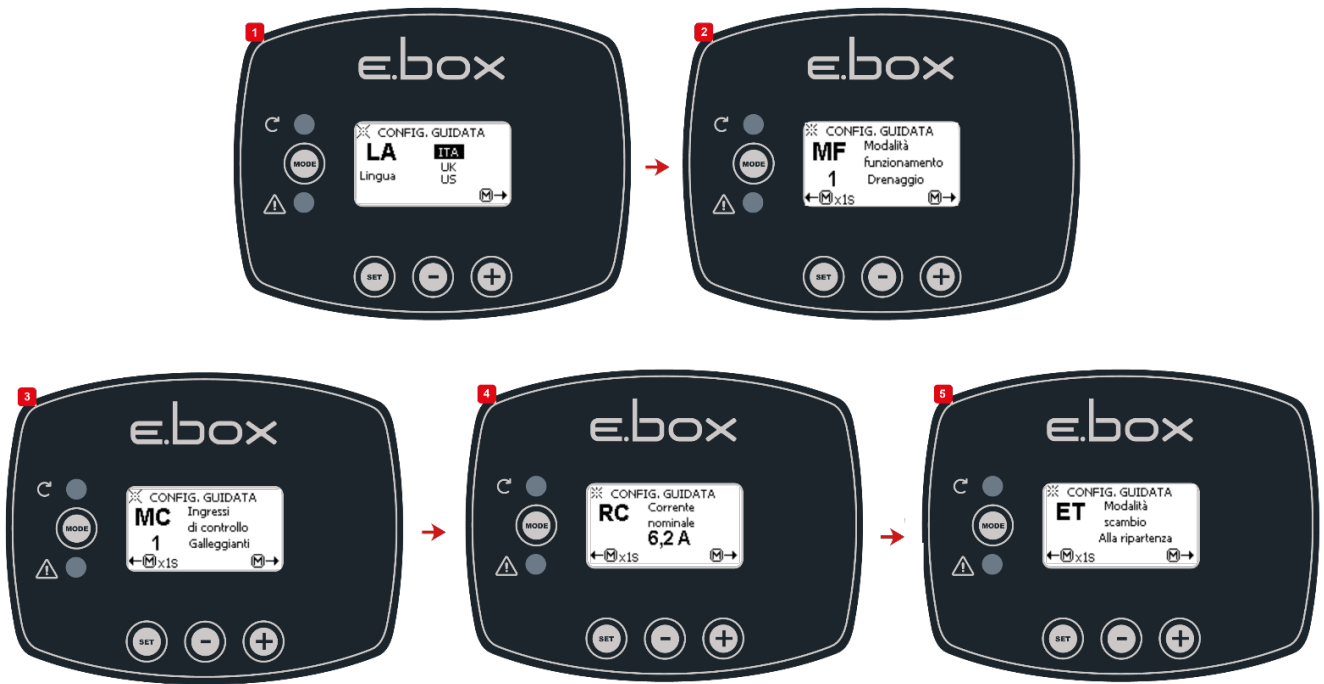
Figure 36: Configuration of Drainage floats or level probes
