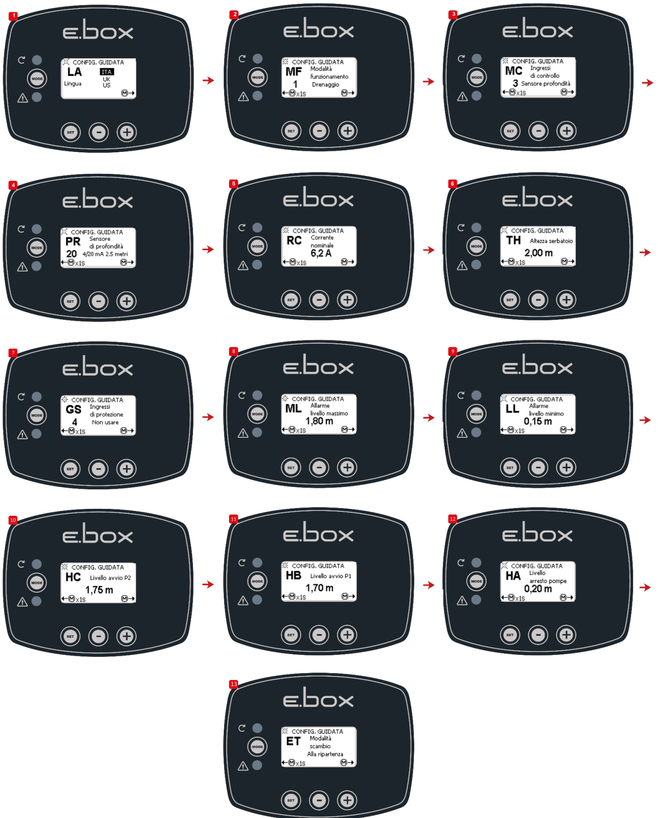
Figure 38: Configuration with only a depth sensor
